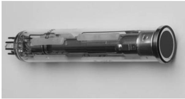
**Figure 2.3.1** Vacuum tube  $\frac{1}{2}$ -in. image sensor.
