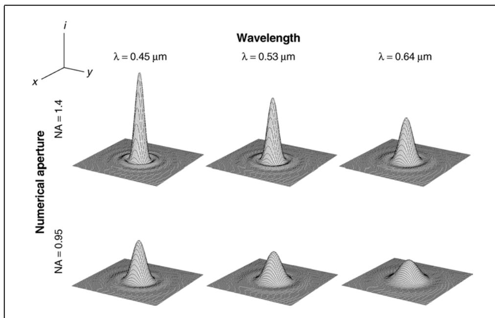
**Figure 12.2.1** Dependence of microscope PSF on numerical aperture (NA, in rows) and wavelength ( $\lambda$ , in columns). Plot coordinates are indicated in the top left corner:  $x, y$  = position (from  $-0.75$  to  $0.75 \mu\text{m}$ );  $i$  = intensity. Width of the PSF decreases with increasing numerical aperture and increases with wavelength.
