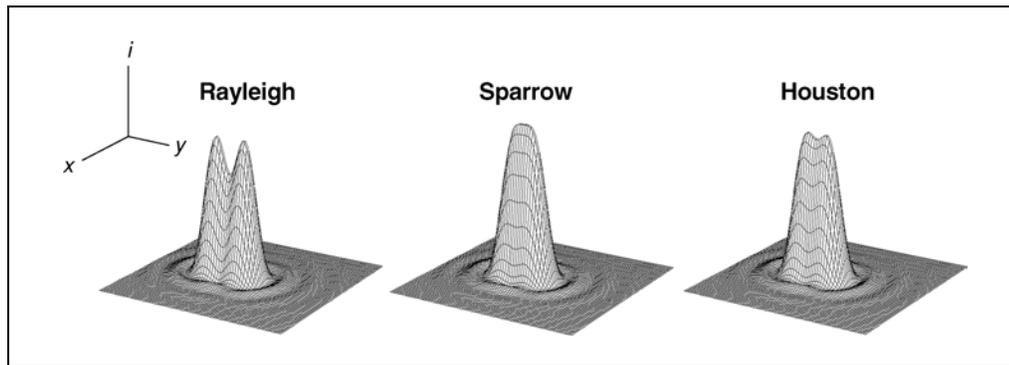
**Figure 12.2.2** Summed image intensities (PSFs) of two points resolved according to (from left to right) Rayleigh, Sparrow, and FWHM (Houston) criteria. Plot coordinates are indicated in the top left corner:  $x, y$  = position (from  $-0.75$  to  $0.75 \mu\text{m}$ );  $i$  = intensity. Resolution (critical distance) depends on what intensity contrast is considered sufficient.
