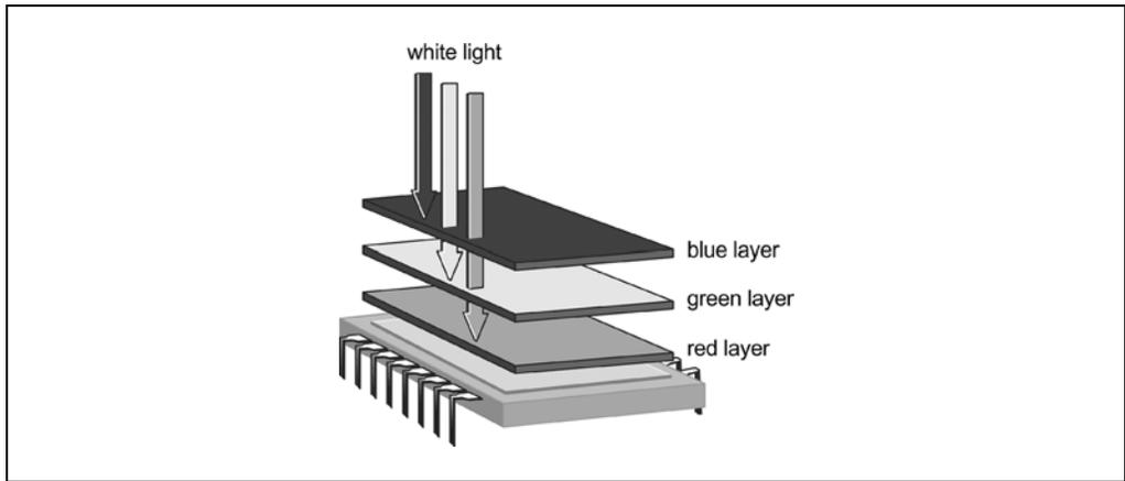
**Figure 12.2.8** Diagram of a Foveon X3 chip (From Foveon Inc.; <http://www.foveon.com>), which filters the color components (RGB) by wavelength-dependent absorption via silicon layers.
