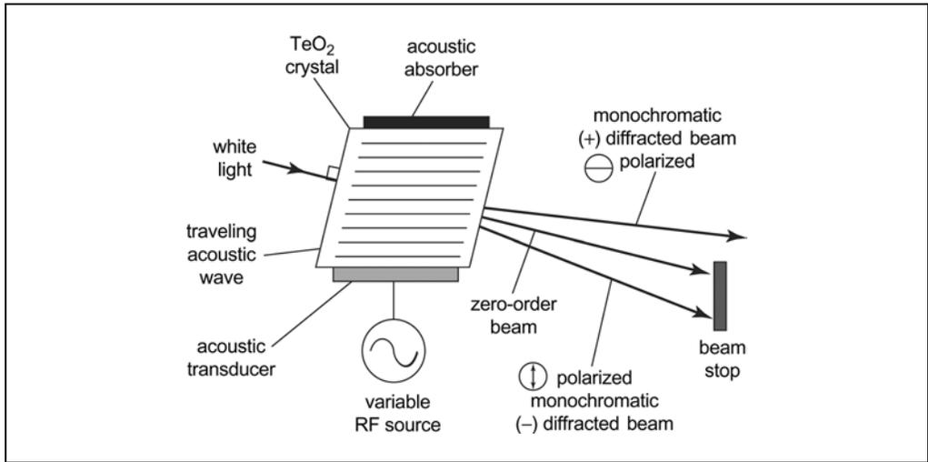
**Figure 12.2.6** Schematic representation of acousto-optic tunable filter (from Brimrose Corp.).
