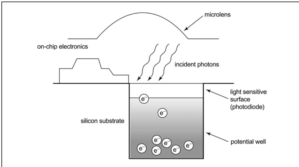
**Figure 12.2.4** Schematic representation of a light-sensitive element (pixel) of a CMOS camera. The photons incident on the light-sensitive area and photoelectrons ( $e^-$ ) trapped in the potential well are indicated.
