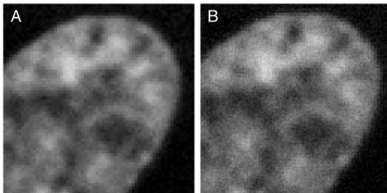
**Figure 12.2.9** Image of AO-stained fibroblast nucleus sampled optimally at the Nyquist rate (2x binning, **A**) and oversampled two times (no binning, **B**).
