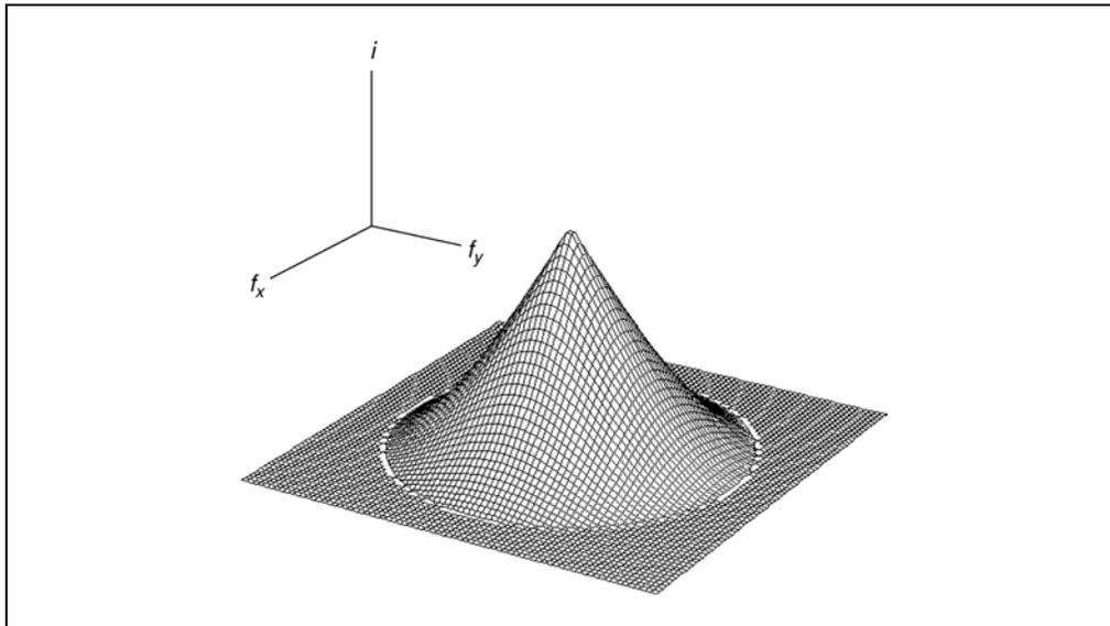
**Figure 12.2.3** Optical transfer function (OTF) corresponding to PSF from Figure 12.2.1 (lower part,  $NA = 0.95$ ;  $\lambda = 0.53 \mu\text{m}$ ). Plot coordinates are indicated in the top left corner:  $f_x, f_y$  = spatial frequencies in  $x$  and  $y$  direction (from  $-4.4$  to  $4.4 \mu\text{m}^{-1}$ );  $i$  = intensity. OTF is 0 above cutoff frequency (i.e., is band-limited).
