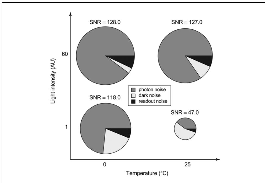
**Figure 12.2.5** Influence of camera chip temperature ( $x$  axis, °C) and incident light intensity ( $y$  axis, arbitrary units) on different components of camera noise. Signal-to-noise ratio (SNR) is indicated by pie size, whereas relative contributions of photon, readout, and dark noise are depicted by pie slices. The parameters were estimated for a Sony ICX085 chip and full well capacity.
