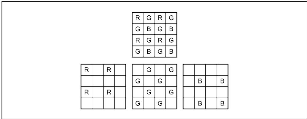
**Figure 12.2.7** Adherent filter matrix (Bayer pattern) comprising red (R), green (G), and blue (B) filters. Top row: the whole matrix. Bottom row: decomposition into color components. Increased sampling intervals in the component images result in lower resolution.
