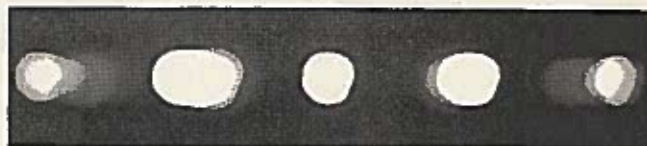
Fig. 6. A photograph of the back focal plane of an objective when a grating on the stage of the microscope is illuminated by a narrow cone of light. The direct light is in the centre of the picture and the diffracted orders of light may be seen on either side. The area which is not illuminated was called the 'dark space'.
