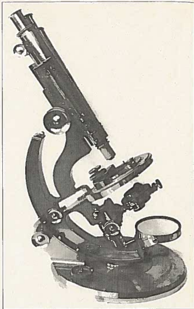
Fig. 3. Ross Radial microscope of the early 1880s. This instrument not only allowed obliquity of substage illumination, but also of the microscope tube itself.
