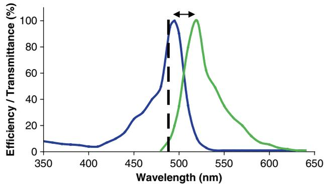
**Fig. 1** Excitation profile (*blue line*) and emission profile (*green line*) of Fluorescein isothiocyanate (FITC) excited with a 488 nm argon laser (*broken line*). Stokes shift is illustrated by the *double arrow*. The long slopes of the excitation spectrum to the blue and of the emission spectrum to the red are clearly visible
