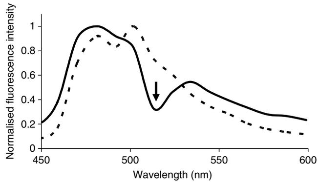
**Fig. 5** Spectral profiles of CFP emission generated from similar wavelength scans to those in Fig. 4a. The profile generated using 458 nm laser excitation and a HFT458 nm main dichroic is shown with a *broken line* whilst the equivalent profile using a HFT458/514 nm main dichroic is shown in a *solid line* and illustrates the drop in fluorescence intensity at 514 nm as the HFT458/514 main dichroic reflects this wavelength (*arrow*)
