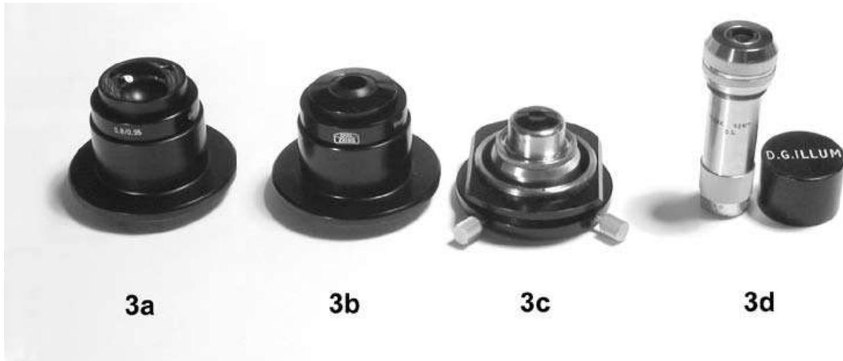
Figure 3. Dark-ground condensers. 3(a) Dry dark-ground condenser. 3(b) & 3(c) Oil-immersion dark-ground condensers. 3(d) Adjustable oil-immersion dark-ground condenser. This condenser can be adjusted to suit different thickness of slide, to give a high quality dark-ground image.
