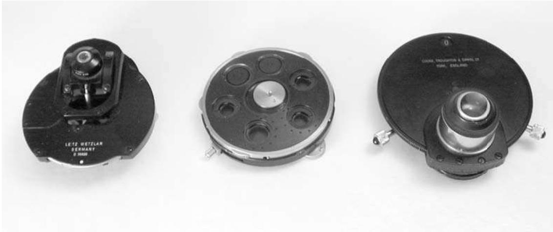
Figure 2. Universal condensers. The central image shows the top cover removed, displaying the revolving disc where the aperture phase annuli, DIC prisms, dark-ground patch stops, Rheinberg discs and Hoffman modulation filters are located. Most universal condensers possess an aperture iris for bright field work, several annuli for phase contrast and a dark-ground stop for low-power dark-ground.
