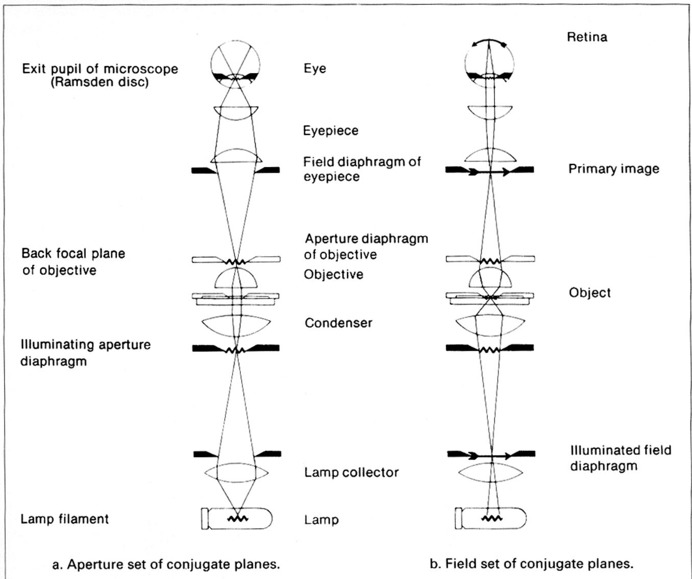
**Fig. 1.** Ray paths of the transmitted-light microscope showing (a) the *aperture* set and (b) the *field* set of conjugate planes. From the RMS Dictionary of Light Microscopy.
