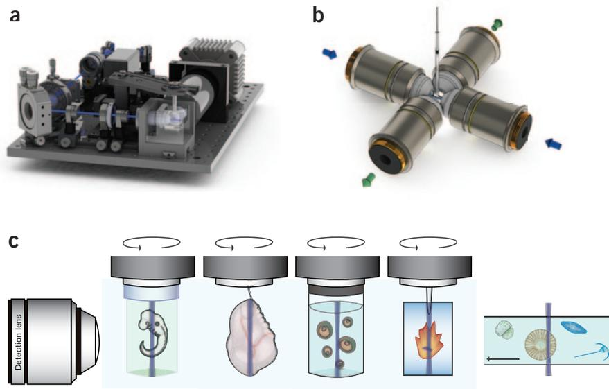
**Figure 2** | (a) 3D rendering of the OpenSPIM design. (b) Schematic of four-lens light-sheet microscope for dual-sided illumination and detection. Image reproduced from Weber, M. & Huisken, J. Omnidirectional microscopy. *Nat. Methods* **9**, 656–657 (2012), Macmillan Publishers Limited. (c) Overview of sample-mounting methods typically used on horizontal multiview SPIM setups: from left to right, embedded, clipped, enclosed, flat and flow-through.
