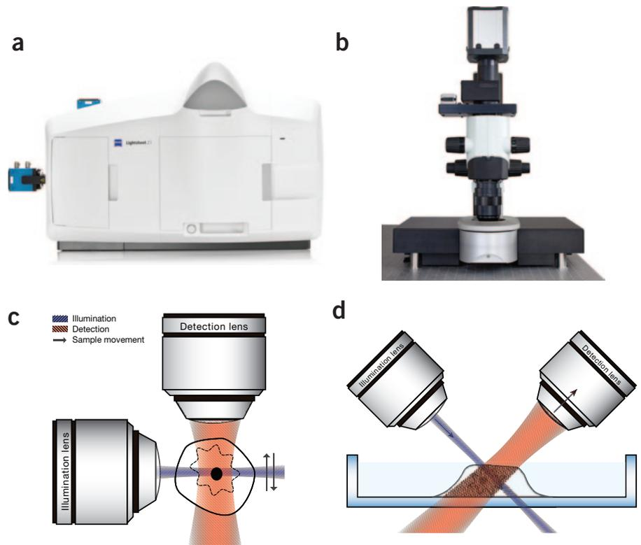
**Figure 1** | Current light-sheet microscopes. (a,b) Available commercial systems are the Lightsheet Z.1 (a) and the Ultramicroscope (b). (c,d) Optical architecture of a typical horizontal orthogonal arrangement in SPIM (c) contrasted with the tilted architecture (for example, iSPIM) (d).
