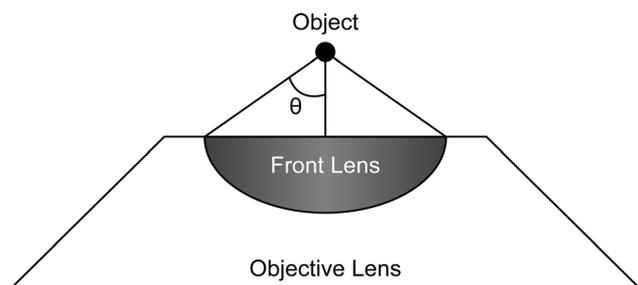
**Figure 2.** Angular Aperture of Objective Lens. The front lens of an objective lens gathers light from the field of view. The amount of light gathered by the lens is described by the angular aperture of the lens, which is defined by the half-angle of light ( $\theta$ ).
