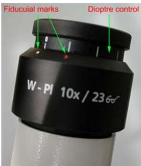
Where a microscope of either type is fitted with one or more eyepieces with built-in focusing adjustments for a photographic frame or a graticule, these should ideally be used in eyepiece tubes of adjustable length, and should be set before step 4. is carried out. For correct adjustment, microscopes having eyepiece tubes of fixed length should always be fitted with a pair of eyepieces with focusing adjustments.
