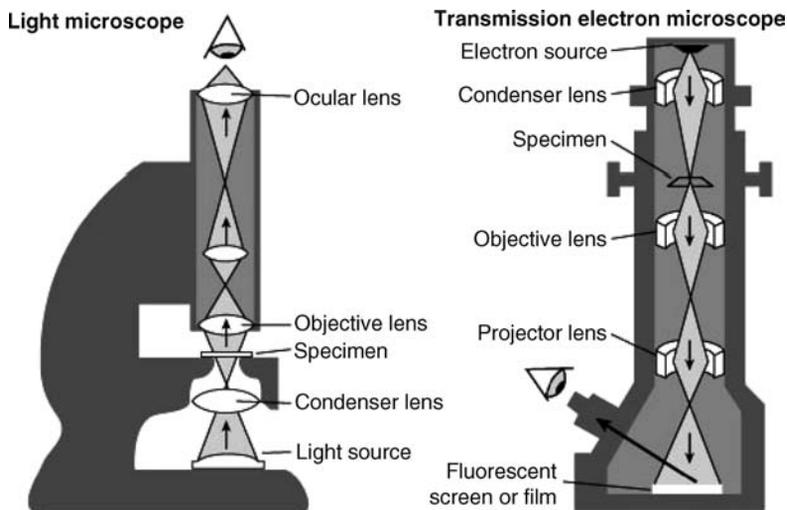
**Figure 7.1** Diagrammatic representation of both the compound light (left) and Transmission Electron (right) microscopes. Blackwell Microbiology Teaching Resources (comparison of electron and light microscopes) © John Wiley & Sons Ltd.
