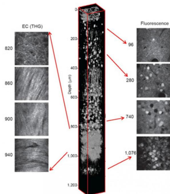
**Xu and his team reveal their new three-photon microscope, which is efficient, doesn’t damage tissue, and can image up to 3.5 millimeters deep into tissue, deep enough to see below the white matter of the brain.** Source: Chris Xu
