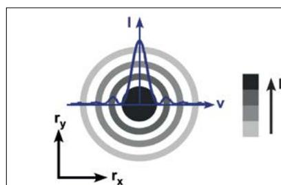
Fig. 1: Due to the diffraction nature of light, a point source will be imaged by a microscopic system as a blurred spot surrounded by rings of decreasing intensities ( $I$ ) in the lateral plane ( $r_x, r_y$ ), the so-called Airy disk (displayed in grey). The intensity distribution along a transverse direction ( $v$ ) is shown in blue.
